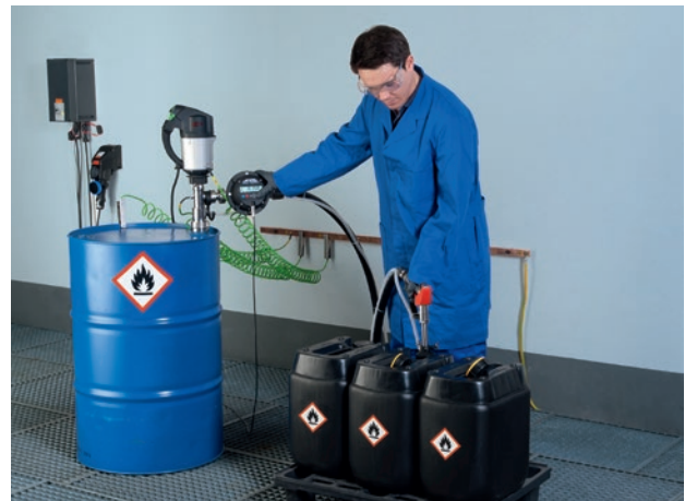
Semi-automatic can filling in explosion zone 1.
