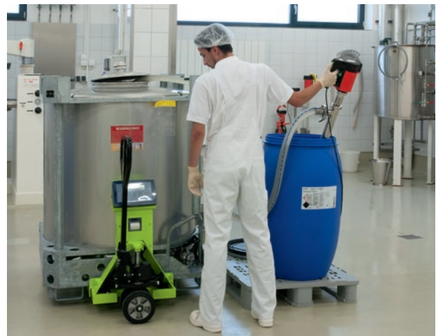
F 560 GS in operation in the hygiene sector – pumping raw material for a cream into a mixing vat.
